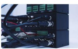
The Hub is a multiplexer module acting as a relay. It is used to expand the system management and the capabilities of your Control Center by enabling control of five additional modules on a single channel. It's a game-changer for operational efficiency.
