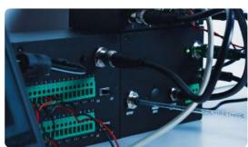
The Advanced Pressure Controller is a single channel pressure controller module with 5 different ranges available (positive and negative pressure from -900 mbar to 8 bar). With the same pneumatic performances as the OB1 pressure controller, run experiments requesting complex pressure profiles and optimum flow control easily.
