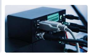
Powerful module with advanced control and communication capabilities for up to 25 modules of the Advanced range. It is a dedicated PLC (programmable logic controller) for microfluidic engineering.
