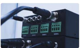
The Sensor Hub is a sensor reader module for up to 4 sensors. It can read all digital sensors from the Elveflow range as well as any 0/10V analog sensors. It is the perfect device for precision monitoring.
