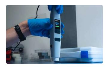
Elveflow's Plasma Bonding Pen is a two-in-one handy tool for optimized surface treatment, ideal for bonding PDMS to glass and PDMS to PDMS. Additionally, it offers advanced surface modification capabilities commonly found in traditional plasma chambers but in a portable and easier-to-use way.
