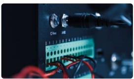
The Valve Hub is a device that can control up to 16 valves. You can configure each group of 8 valves to either be supplied by 24V signals or by 12V signals.
